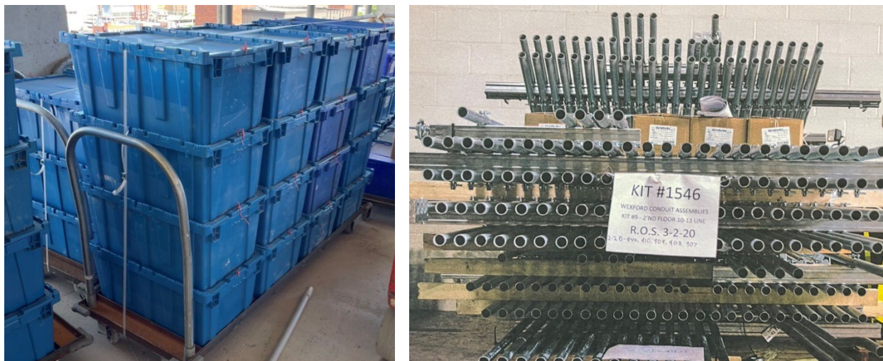
Figure 8: Kitting (left) and prefabricated racks (right) ready for shipping and installation.
